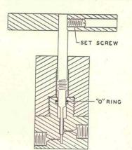
Fig. 1. "O" ring high pressure valve.
